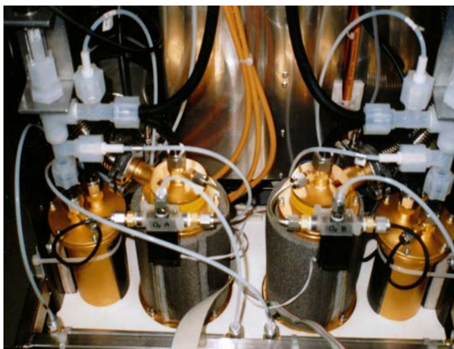
CLD 790 SR - 2: A Golden Standard. Reaction chambers.
